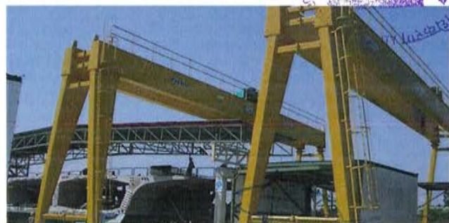
Figure 11: Rail Gantry Crane Lifting Arrangement
