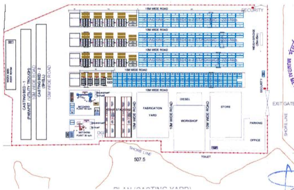
Figure 5: Casting Yard - Concept Layout Plan
