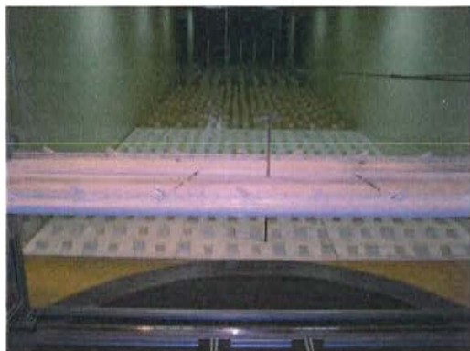
Wind stability of bridge deck
