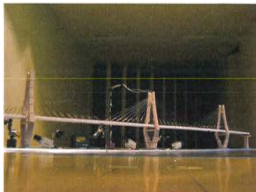
Bridge full model wind test
