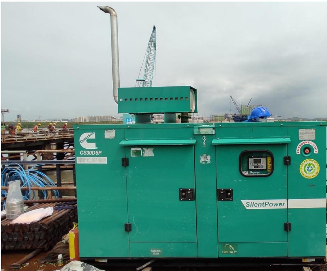
**Photographic evidences of construction equipment used by contractors are provided with exhaust silencers to reduce noise**
