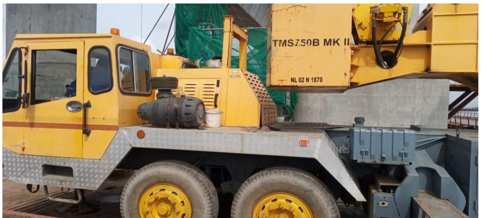
**Photographic evidences of construction equipment used by contractors are provided with exhaust silencers to reduce noise**
