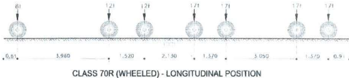
Figure 5-5 Class 70R Wheeled vehicle. Axle loads and longitudinal arrangement (dimensions in m).
