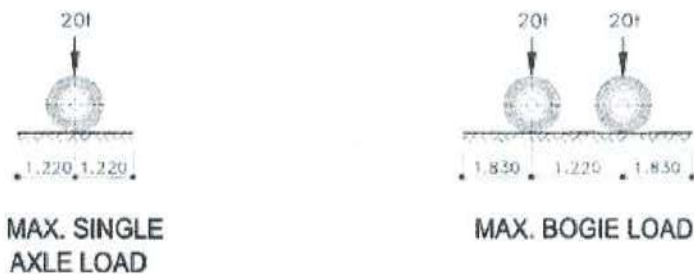
Figure 5-6 Class 70R Wheeled vehicle. Axle and bogie loading (dimensions in m).
