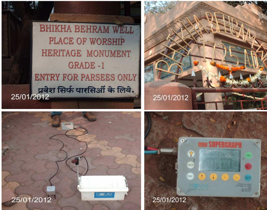
The graph has been plotted for radial, transverse and vertical vibration and shown in **Figure 3.46**, **Figure 3.47** & **Figure 3.48** respectively. The result of the monitoring shows that, the average radial vibration is about 86 VdB and the peak radial vibration is 88 VdB. The average transverse vibration is found to be 81 VdB and the peak transverse vibration is 83 VdB. The average vertical vibration is 107 VdB and the peak vertical vibration is found to be **113.9 VdB**.
