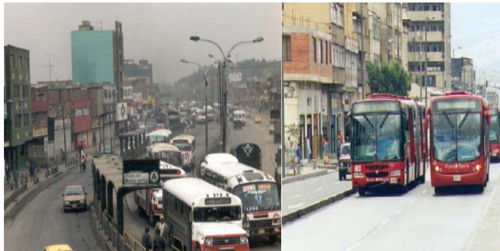
Figure 4.3 :Bogota originally operated an open system that created congestion (left), whereas operating a closed system has proven to dramatically improve travel times and customer comfort (right).
