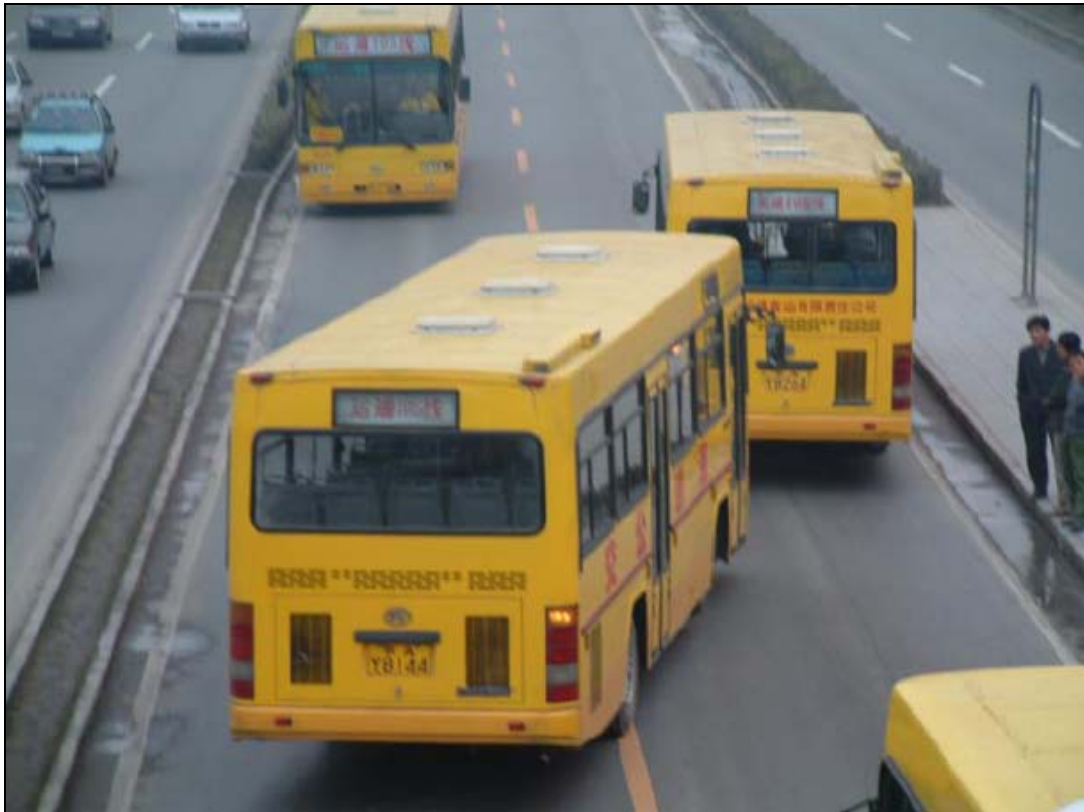
Figure 4.5 : By allowing vehicles to overtake in the opposing lane, there are obvious risk of serious collision as evidenced in Beijing
